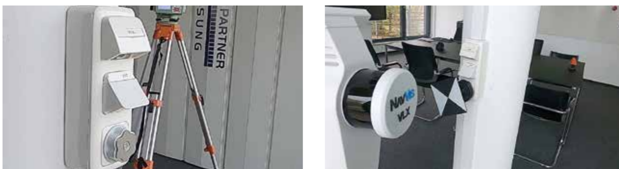
The image shows the use of the targets in combination with a NavVis instrument. Reference points for sockets RSFP-X90-30 to 36 and the suction cup RSSV-X90 are particularly very popular for indoor applications. You can find a related video on our YouTube channel.
